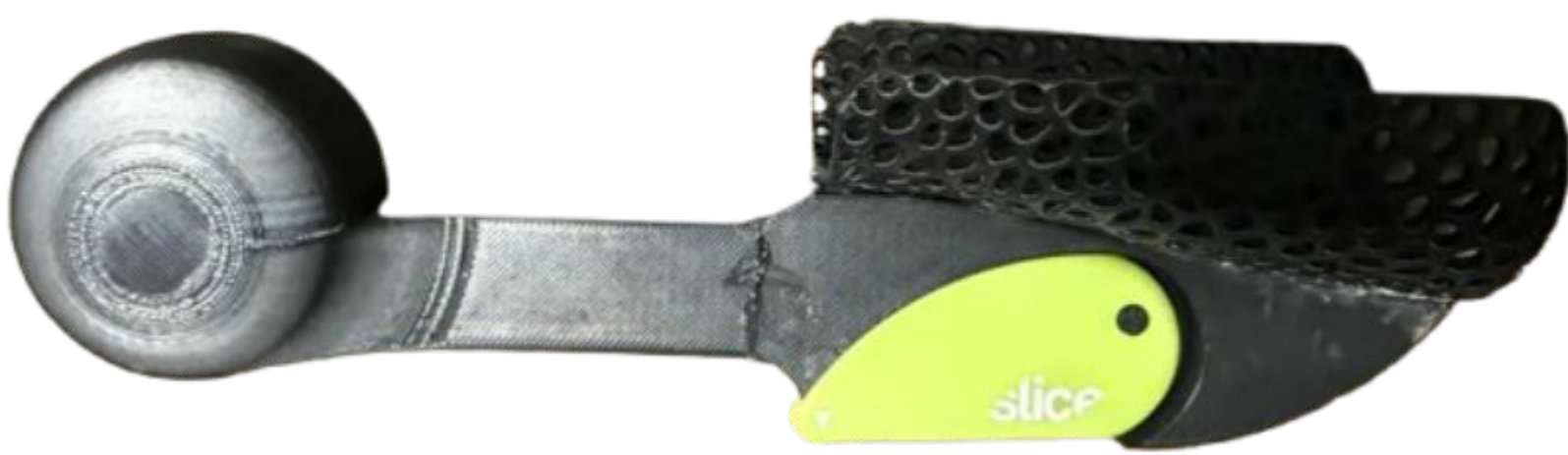
Fig.2 Side profile of PLA 3D printed devices with integrated blade attached under the wrist rest
